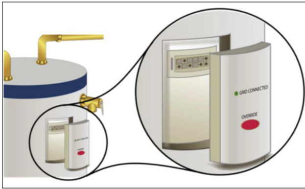
Figure 1: Illustration of CTA-2045 Port on a Water Heater, and a CTA-2045 AC Form Factor Communications Module. Figure modified from EPRI
